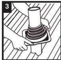
3 Slide flashing over Pipe using water.
